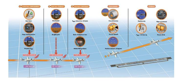
If the pilot is not within parameters at the 1,000-foot or 500-foot gate and doesn't believe he can correct the situation before the next gate, he should go around. If out of parameters at 200 feet, go around. *Illustration by Charles Floyd*
